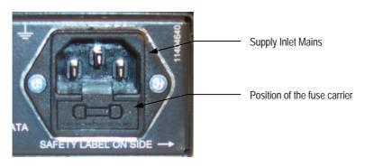
Figure 2.2: AC Power Inlet Assembly
